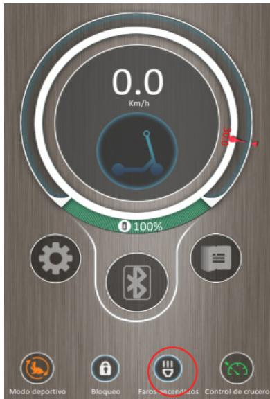
You can turn on or off the front light of the e-scooter via your smartphone. When the icon of the front light of the application lights, it shows that the light is on, if the icon is not lit, the front light of the e-scooter is off.
