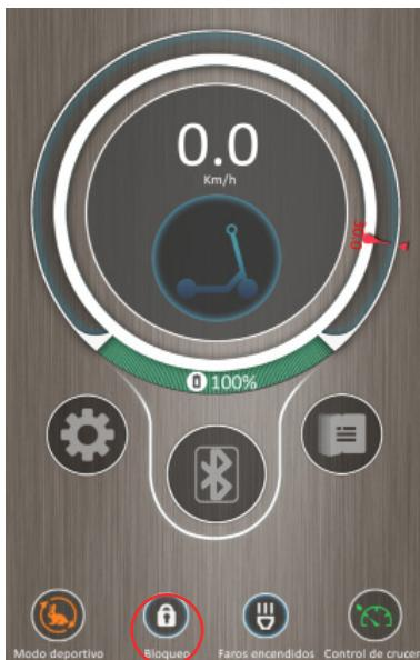
When the lock icon is illuminated (deadbolt closed), the scooter locks, when it does not light, show unlocking (open bolt).
