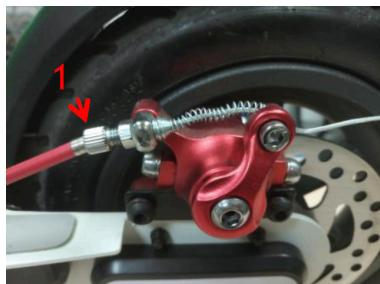
**2.** Turning the adjustment 2 brings the piece 4 closer to the disc. This adjustment can be done with the Allen key provided with the equipment.
